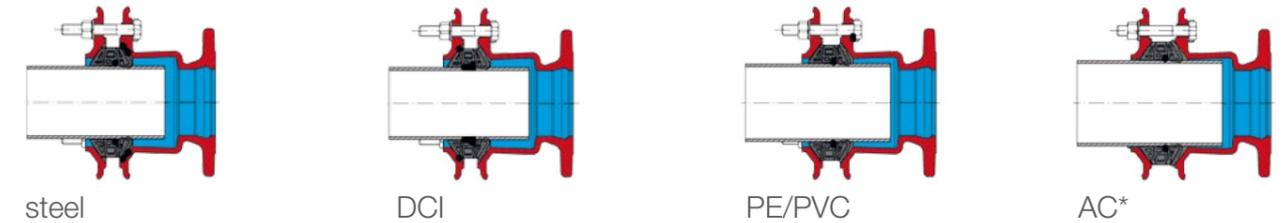
\* Warning! A restraint connection between Synoflex and asbestos cement pipes can't be confirmed. Removal of the grip ring is not necessary.
