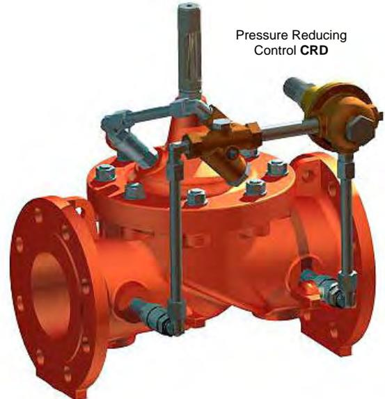
The CLA-VAL SERIES 90 reduces a higher inlet pressure to a constant downstream pressure (Pressure Reducing Control) regardless of changing flow rate and/or varying inlet pressure.
