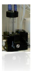
Photometric measuring cell complete with RS485 serial interface card
