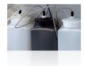
Continuous monitoring of the reagents through level probes. The powder DPD reagent to be diluted before use is an excellent solution for storing the product safely in any place.
