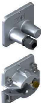
**Turret** – Cast aluminium twin turret allows cable sealing using heat shrink tubing. Maximum cable diameter 20mm.
