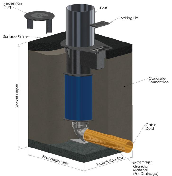
See **RS socket** installation guide for EN40-3-1:2000 foundation guidelines
