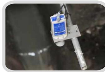
The Cello CSO Level recorder has sophisticated alarm regimes for detecting and immediately signalling abnormal conditions. These include high & low alarms levels as well as profile alarms. The Cello also reports in-situ signal strength, GSM network errors and low battery levels
