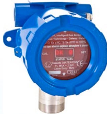
The Monicon S500L-IR-N2O is a high quality, self contained, NDIR (Non Dispersive Infra Red) gas monitor that offers a host of sophisticated features to provide fast, reliable warnings against dangerous concentrations of nitrous oxide gas.
