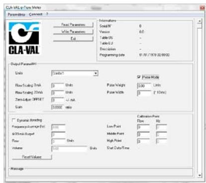
**Programming:** CLA-VAL software can easily configure the type and size of the valve in which e-FlowMeter is inserted.
