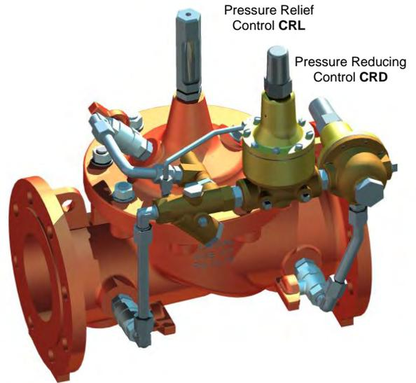
The CLA-VAL SERIES 90 reduces a higher inlet pressure to a constant downstream pressure (Pressure Reducing Control) regardless of changing flow rate and/or varying inlet pressure.
