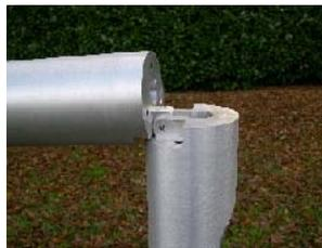
9. Carefully walk backwards during lowering, with both hands high onto the column, to decrease the top weight.
