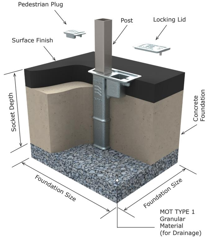
See **RS socket** installation guide for foundation guidelines
