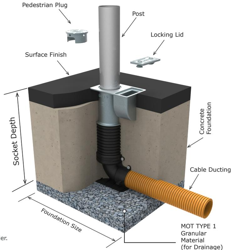
See **RS socket** installation guide for EN40-3-1:2000 foundation guidelines
