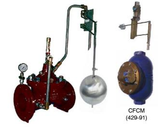
The CLA-VAL SERIES 420 Modulating Float Level Control Valve maintains a constant water level in a reservoir by compensating for variations in supply or demand. It can be installed to control the flow into or out of the reservoir by closing on rising level or opening on decreasing level.
