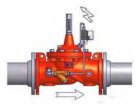
The CLA-VAL SERIES 136E/D Solenoid Control Valve is an On/Off Control Valve which either opens or closes upon receiving an electrical signal to the solenoid pilot control.
