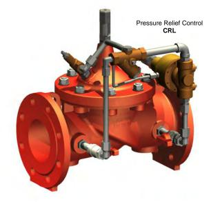
The CLA-VAL SERIES 50 Sustaining Valve accurately maintains a minimum preset (Pressure Relief Control) inlet pressure regardless of changing flow rate. The CLA-VAL SERIES 50 Relief Valve opens fast to dissipate excess system pressure.
