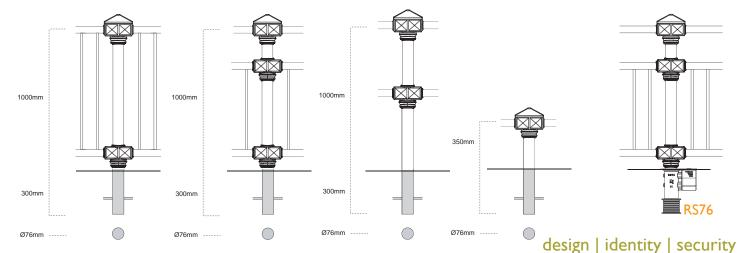
Moy railing (code) I bar full guard ¾ guard 2 bar Height (above ground): I000mm I000mm I000mm 350mm (Panel lengths 2M / I.5M / IM available) Depth (below ground): 300mm 300mm 300mm 300mm Diameter (core post) Ø76mm Ø76mm Ø76mm Ø76mm Total Weight: n/a n/a RS76×300 RS76x300 RS76x300 RS76x300 RS socket option:
