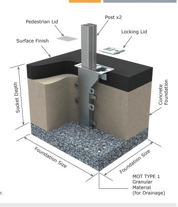
See **RS socket** installation guide for foundation guidelines For detailed foundation sizing on specific site conditions contact your supplier.
