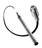
The MJK Expert™ Log 900 Level Logger is battery powered with a built-in data logger. It is designed for level and temperature recordings in wells, bore holes and storm flow locations over longer periods. It has an external diameter of 22 mm and is made of 316L stainless steel.
