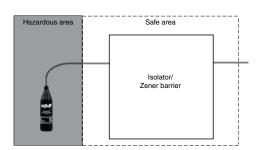
When using model Expert™ level transmitters 1400/3400 in explosion hazardous environments Category 2 (Zone 1 and 2), an isolator or a zener barrier must be used.
