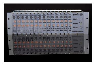
The Monicon Multichannel Gas Monitor is an innovative, cost effective, rack mounted system. Two control cards are available. Part number C25005 is designed for use with the T100 detector head while Part number C55005 control card is designed for use with the CGS500 or similar thermocatalytic sensor.
