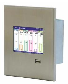
**Panel or in-wall mount MultiCon CMC-99SL** is featured by a shallow casing - only 55 mm! All connectors are introduced on side walls of the device as in a typical panel computer. As the number of measurement inputs and outputs is limited, this design in intended mainly for systems with a small number of signals or systems which include other measurement systems with Modbus RTU interface. An Ethernet interface is also available to upgrade every MultiCon control's application easily.
